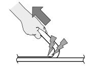
Do not separate the channel at the gap of mounting base.
