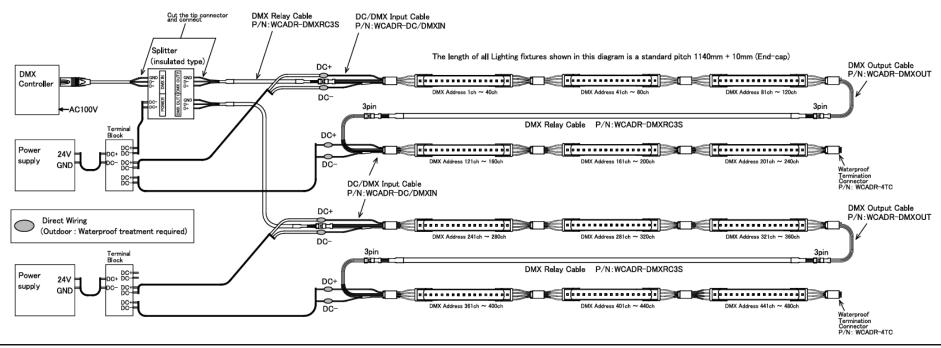
2) In the case of a connected fixture length of 5m or more (exceeding the maximum series connection length)
