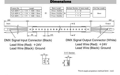
When connecting products and power supplies in parallel in multiple systems, make sure that the types and lengths of the wires in each system are the same to prevent differences in brightness and color between the products
