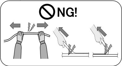
Do not separate the mounting channels at the gap (joint parts) between mounting bases.
