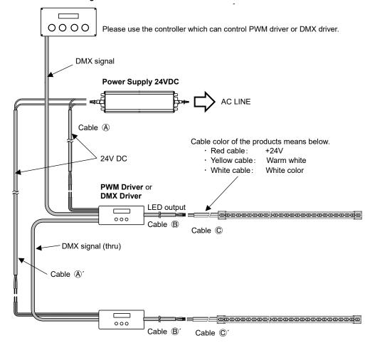
• Divide the wiring in parallel not to exceed the "Maximum series connection length" and the "Limits of current value and wires".
