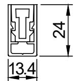
Cross-sectional sizes when installed with FAC20-01GD / FAS00-01GD
