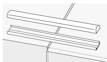
The channel can suppress vibration and misalignment of the base, and prevents the break of the product.
