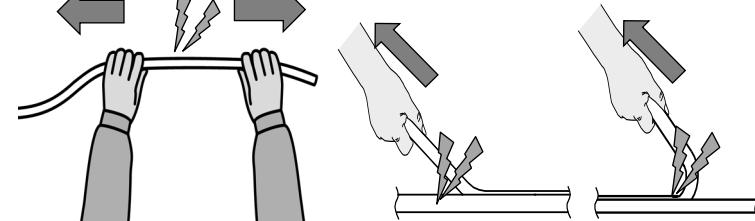
Do not separate the mounting channels at the gap (joint parts) between mounting bases.
