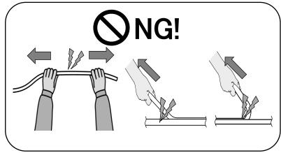
Do not separate the channel at the gap of mounting base.
