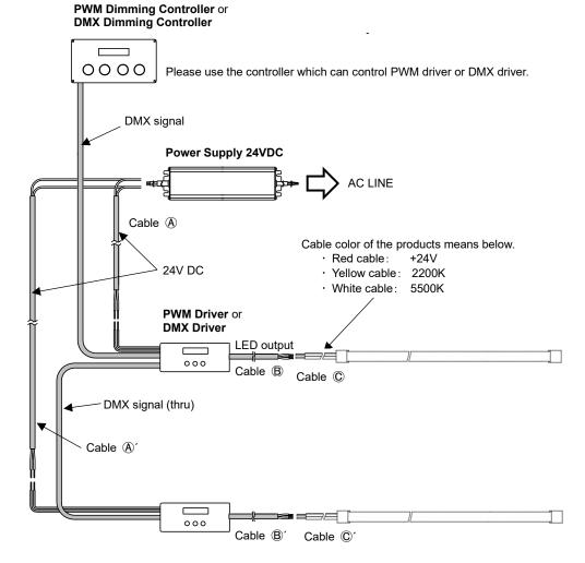
• Divide the wiring in parallel not to exceed the "Maximum series connection length" and the "Limits of current value and wires".
